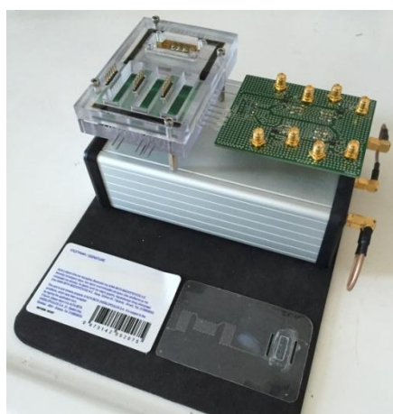
Foodborn Bacteria detection device developed in the framework of the FP7 funded European program LoveFood. The plastic cartridge on the bottom right part of the figure, equal to the size of a credit card, is used for the loading and analysis of the sample.
