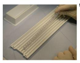
5 Keeping the right side of the frame slightly elevated, place the left side of the frame against the mechanical stop (about 2 cm, or 1 inch, from the end of the tray).
