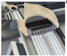
**20** Select the fixed electrode [Anode] (see Figure 4 in Section 1 of the *Agilent 3100 User Manual*) and place the two tabs on the electrode into the slots on the left side of the tray. Rotate the fixed electrode down into position over the electrode pad (insert). Push down until the fixed electrode clicks into place. Slide the tray without lifting it into the anode connector.
