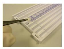
**13** Place a second wetted electrode pad on top of the first electrode pad. Each end of IPG strip should now be covered by 2 pads each which are on top of each other.
