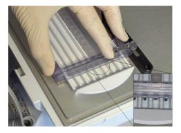
**21** Insert the moveable electrode [Cathode] (Figure 4 in Section 1 of the *Agilent 3100 User Manual*) in the orientation shown and push down until it clicks in place. (Lane labels on the electrode should read **A-H** on the right side with **A** at the top of the electrode.)
