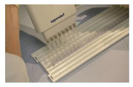
**7** Pipette 40 μL of IPG Strip Rehydration Solution into each of the wells.
