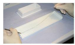
3 Place the IPG strip in the tray with the gel side up.Observe correct tray orientation with handle on the right and fixed electrode slots on the left.
