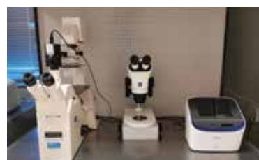
Fig. 2: Dissection hood containing a stereo microscope, Zeiss imaging system and the Countess III automated cell counter.
