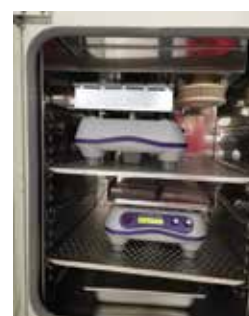
Fig. 4: CO 2 incubator for culturing of forebrain organoids, including shaking platforms.
