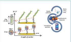
Left: measuring the size of a protein and a DNA molecule through acoustic sensing; Right: 3D-printed point-of-care platform for genetic testing of infectious diseases directly in human samples using an acoustic sensor and a smartphone
