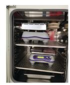
Fig. 4: Co<sub>2</sub> incubator for culturing of forebrain organoids, including shaking platforms.
